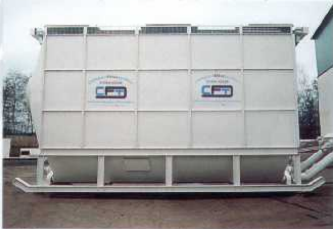
Semi-mobile de-dusting units 120,000 m 3 /h
